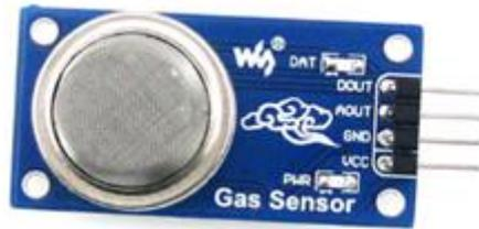
Gambar 3. MQ-2 Gas Sensor
