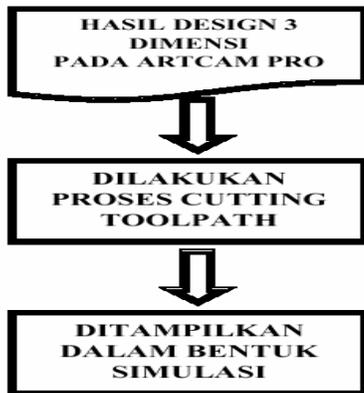
Gambar 2. Proses toolpath
